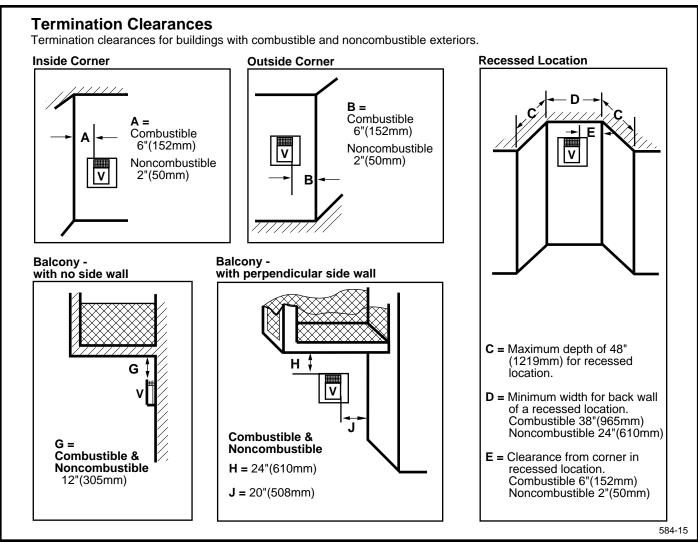
Fig. 10 Termination clearances.
